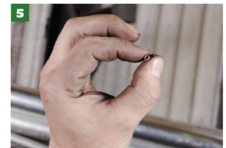
**5** Remove the smaller pilot jets with a good fitting flat bladed screwdriver. These only need to be checked for dirt or blockages so hold them up to light and check. Clean through carefully with the strand of a wire brush if it needs it.
