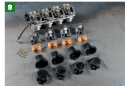
At this stage carefully check each of the parts you have removed for damage, particularly on the rubber diaphragms which need to be in good condition. The smallest of rips or tears here causes big problems as the vacuum will be lost.
