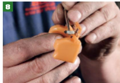
Inspect the end rubber seals for damage as they stop fuel from seeping through when the engine isn't running. If fuel pressure is higher than 3 psi this is where they will leak from.
