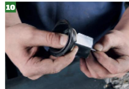
Next the needles to be inspected. Carefully remove them from the diaphragm by using your thumb to cover the top of the needle, as it houses a small spring that can easily shoot off, so very slowly feed the needle through from the bottom.
