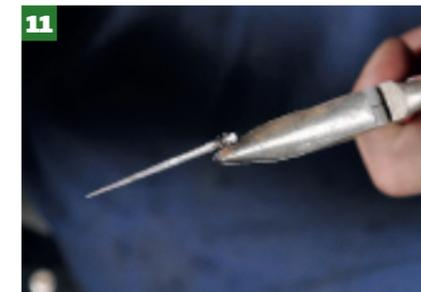
Remove the push-on spring and bush from the top of the needle. Check that the circlip is on the middle locating groove on each of the needles. Carefully refit the needle back into the diaphragm. Not all carbs have adjustable grooved needles.
