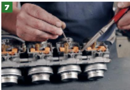
Carefully remove the floats. On these R1 carbs they are held on with a sliding pin but other makes of carbs have different designs such as small bolts keeping them in place.
