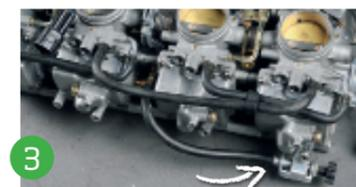
3 For tickover adjustment, there is a screw that is often remotely housed on a cable that is linked to just one carb. This is the master carb, which controls the other carbs and will adjust the position of the butterfly to those simultaneously. In order to balance them, a carb vacuum gauge is needed to take a reading off just the master carb, the others do not need to be touched.
