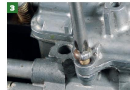
3 Flip the carbs over then unscrew and remove the float bowls. Again be careful to use the correct sized screwdriver. Clean the bowls out carefully to remove any residue from petrol or dirt that may be in there.
