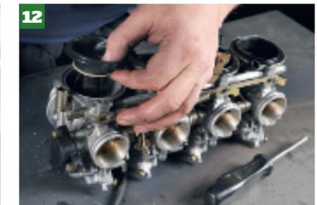
There's no need to strip them down any further, so once all of the parts are properly cleaned and inspected for damage or dirt then reassembly can begin. Locating lugs on the diaphragm covers ensure you can't get it wrong but take your time.
