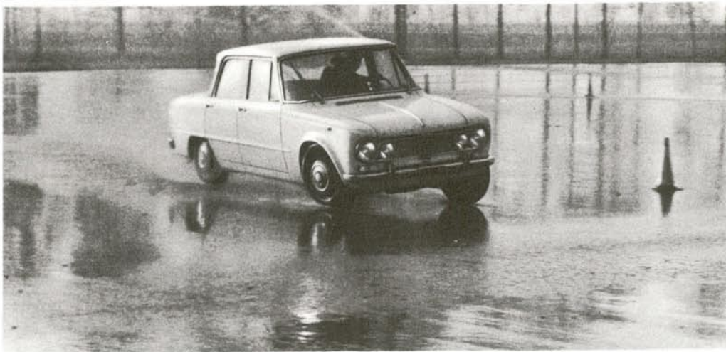
THE GIULIA CORRECTING A CURVE - Even on a wet road. The cornering ability is being tested on an enormous circular track made of various types of asphalt which has been artificially flooded.
