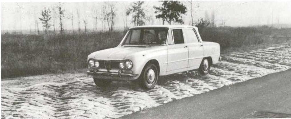
ON COBBLES - Difficult, merciless tests for the suspension and shock-absorbers are purposely carried out on surfaces much rougher than any in existence in order to discover more rapidly the limits of endurance.
