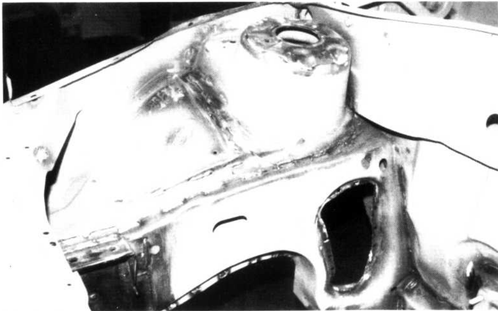
The completed inner wing — note 'stitch welding'
