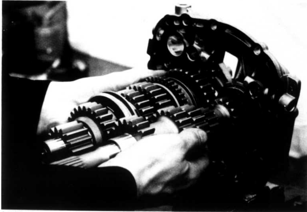
Introducing the shafts onto the sandwich plate
