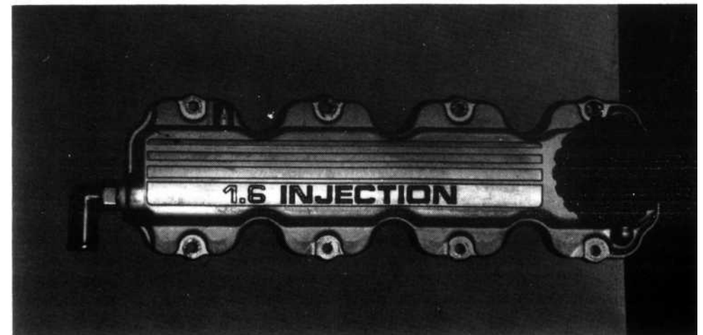
The new external breather connector
